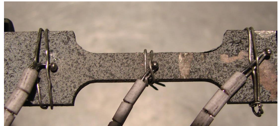
SS316/T22 DMW sample image after 378 hours creep testing
